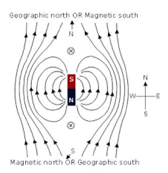
**RESULT:** - The magnetic lines of force of the given bar magnet is shown on the white sheet of paper.
