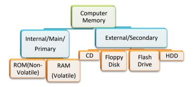
**(Storage Devices)**—There are two types of storage devices used with computers: a primary storage device, such as RAM, and a secondary storage device, such as a hard drive. Secondary storage can be removable, internal, or external.
